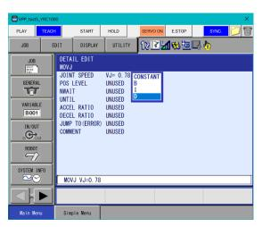
3. Select enter to record the position...using a variable for a set speed.
